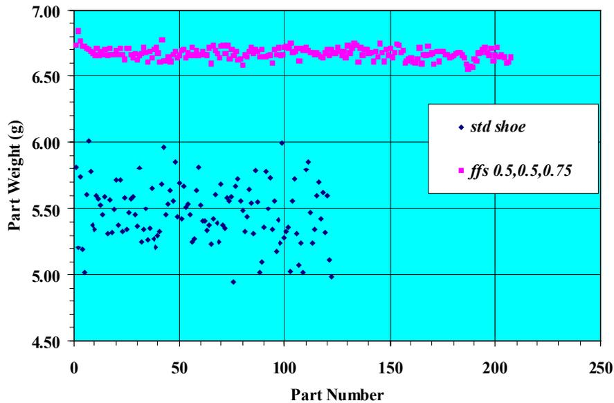
(b) Weight control for poorly-flowable iron alloy
