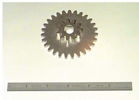
**(b) Two-level sprocket gear**
